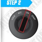
Turn Key to Aux/On position (just short of cranking - Don't crank)
